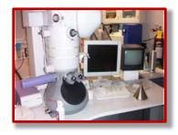
dispersive X-ray spectroscopy (EDX). Using the TEM as electron probe nano-analyzer will provide users with immensely important data to assess the behavior of the actinide metals in fresh fuel with unmatched spatial resolution.
